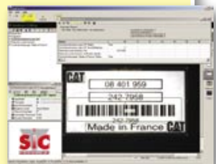
Identification tag inspection
